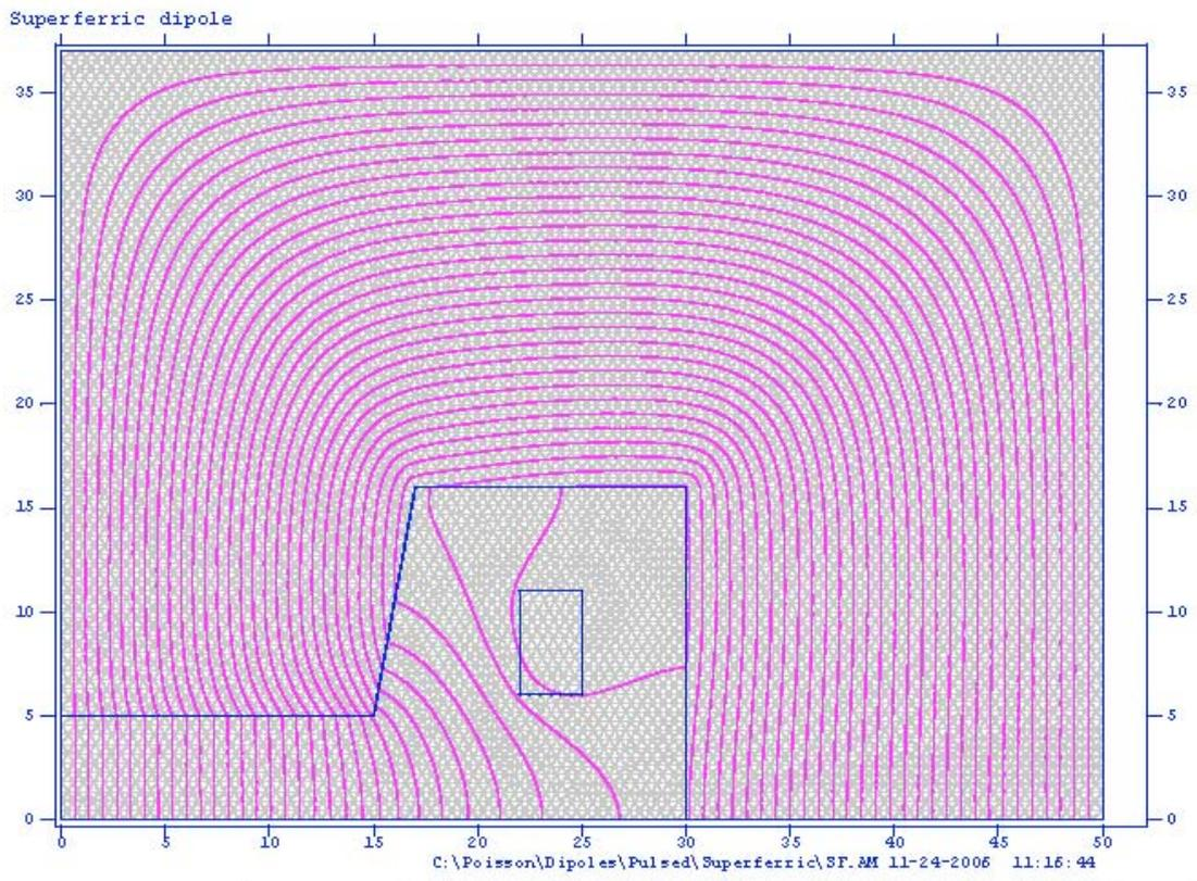
Fig. 4 Cross-section of the superferric dipole for PS2 (W. Scandale)
