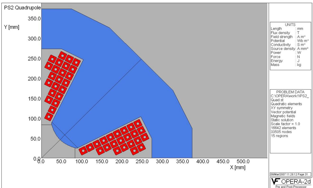
Fig. 3 Cross-section of the normal conducting quadrupole for PS2 (T. Zickler)
