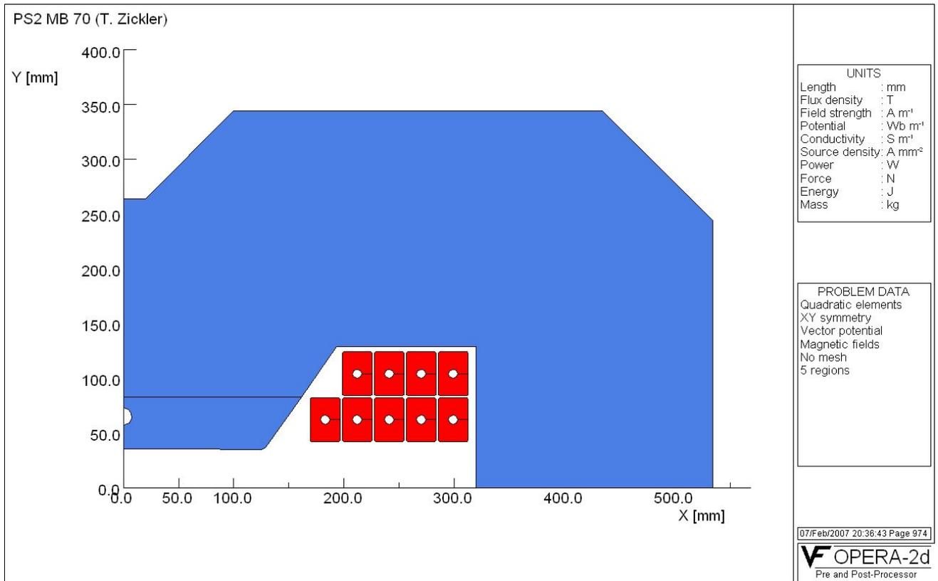
Fig. 2 Cross-section of the normal conducting dipole for PS2 (T. Zickler)
